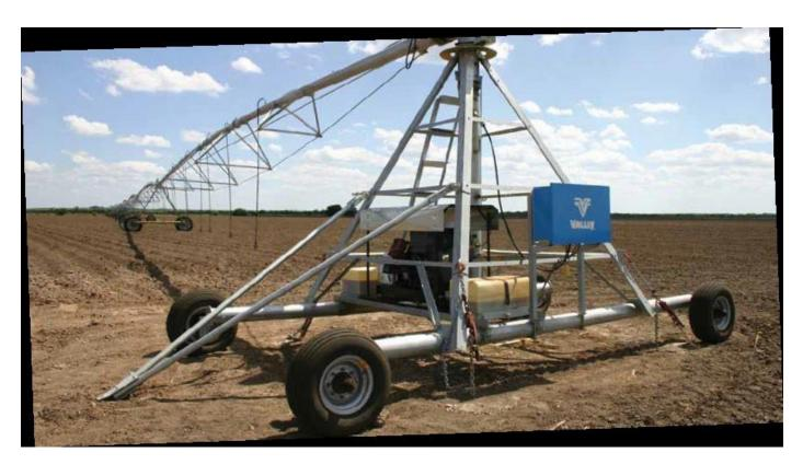
Valley towable options allow you to irrigate two or more fields with one machine to reduce your installed cost per acre. Each towable machine can be towed from one field to another in less than an hour. You can choose from an on-board engine generator or public power supply to power your machine.
